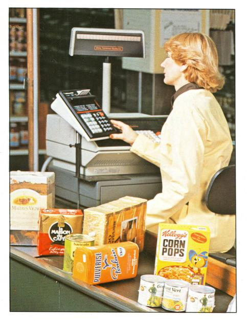
A keyboard of the kind of a cashregister, which may be equipped with up to 15 function keys. This is used by the shop staff to initialise the terminal, to open and close the device, to consult the log store and to communicate with the inter-bank data processing system.
