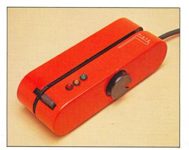
The DEBIMAT 200 also accepts payment cards with standardized magnetic stripes. To this end, one needs only to supply the vendor's module with a specialized card reader, the LCPM model 203 M, which can read standard magnetic stripes (ISO/2/3554).
